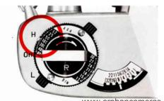
The "H" and "L" marks alongside the flange surrounding the rewind crank are control settings for the CdS exposure meter and indicate the meter's high and low sensitive ranges. On this flange is a line that should be set opposite to "H" or "L" depending on the prevailing light situation.
