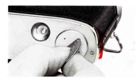
The mercury battery is housed in a special compartment in the base of the camera. Access to the compartment is provided by a round, screwout cap.
