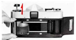
When the film is completely rewound into the cassette, open the back cover by sliding the Back Cover Release Lever to the "O" position. Pull up the rewind crank shaft and remove cassette.
