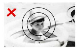
When the scene is out of focus it will appear as shown in the picture on the left. If the scene seen through the viewfinder cannot be brought into clear focus after turning Focusing Ring in both directions, the subject is outside of near limit of camera's focusing range. Use extension tubes to bring subject into focus.
