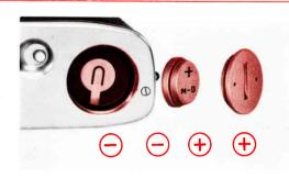
To replace battery unscrew cap, take out old battery and replace with new one, being careful to observe polarity marking. +(plus) polarity marking on new battery should face out, toward the battery compartment cap, and - (minus) toward camera.
