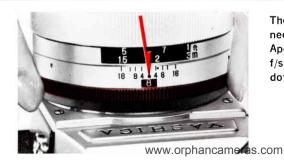
The f/stop number shown by the needle is then set by turning the Aperture Control Ring until this f/stop number is opposite the red dot.
