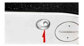
Press the Film Rewind Release Button which is located on the base of the camera. The Film Rewind Release Button should be kept depressed while the film is being rewound.
