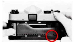
Advance the film with one stroke of the Advance Lever, and make sure the perforations in the film are threaded on sprocket teeth.
