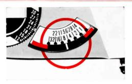
Aim the camera at the subject, the red indicator needle in the Exposure Meter will then show the proper f/stop number.
