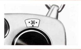
After taking a full roll of film, it is necessary to rewind the film into the cassette before removing the exposed film from the camera.
